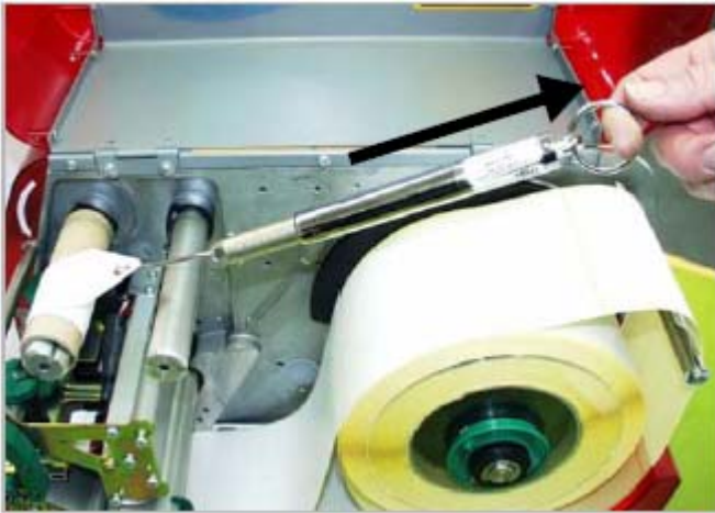
[23] Measuring the brake force at the ribbon rewinding mandrel
