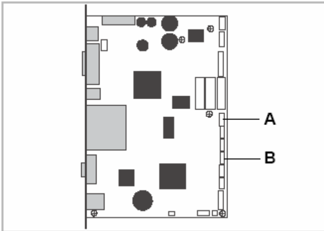
[40] Sockets for the punch sensors on the CPU board A Transmission sensor (CN905) A Reflex sensor (CN 908)
