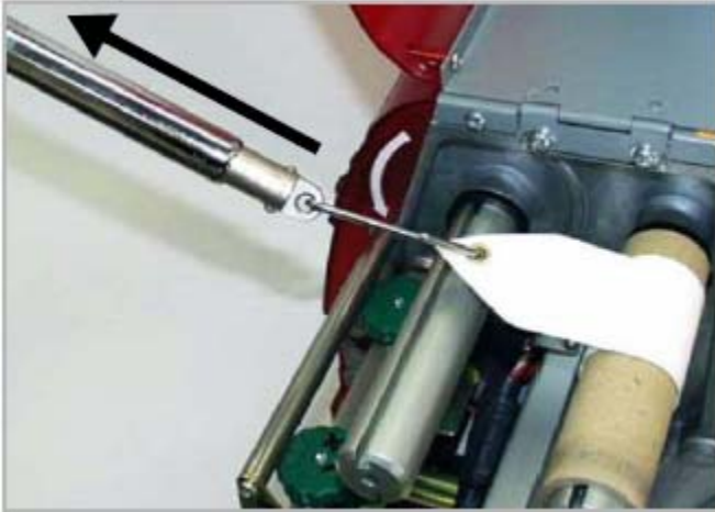
[14] Measuring the brake force at the ribbon unwinding mandrel
